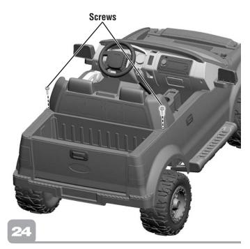
Insert two screws through the back of the seat and into the vehicle. Tighten the screws.
